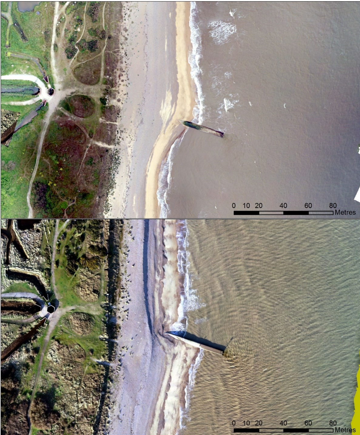
Figure 1: Downtide erosion and updrift accretion resulting from the partial blockage to longshore sediment transport caused by the Minsmere Sluice Outfall following NE (top) and SSE (bottom) storm conditions.
